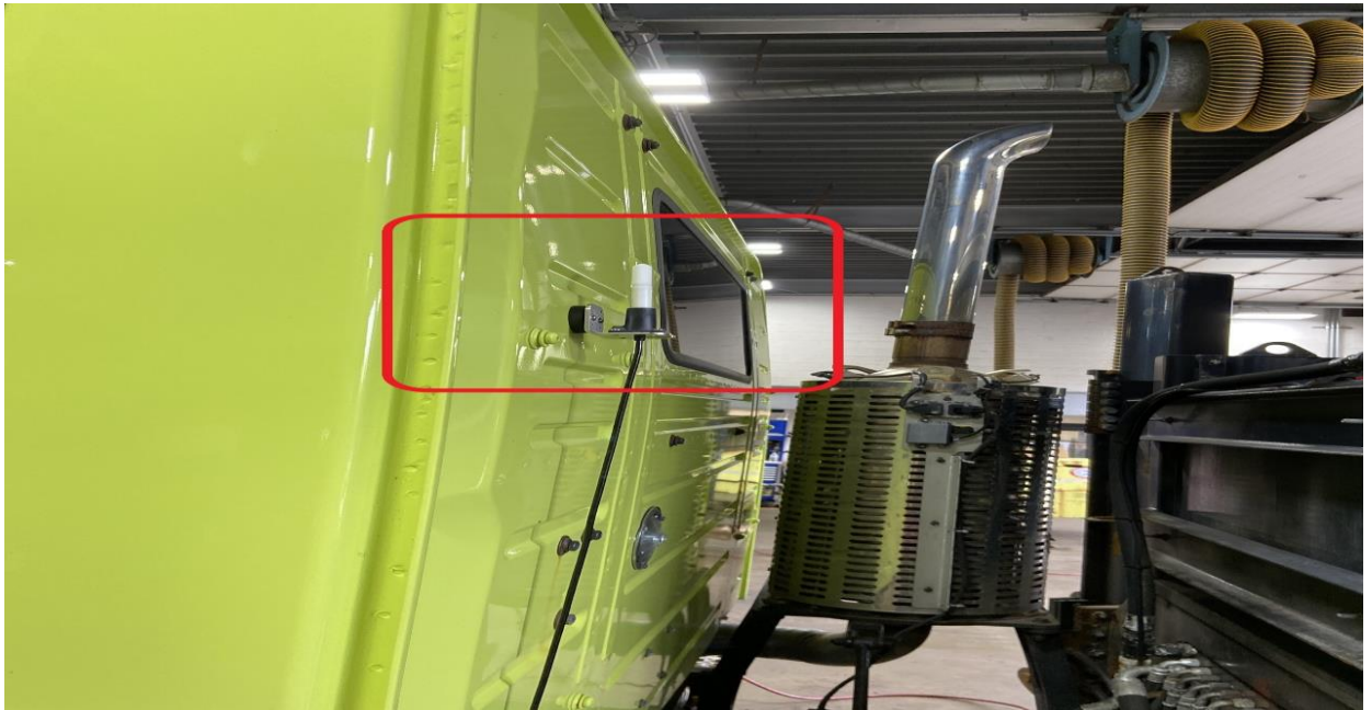
Figure 8. Air temperature and humidity (ambient weather) sensor installed at the back of the cab on a plow truck
