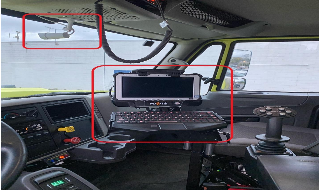
Figure 9. Windshield camera and the tablet computer installed in the cab of a plow truck
